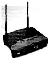
A wireless router is a device which allows computers to communicate via radio waves
